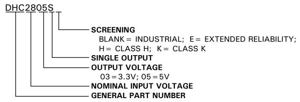
The above example is an industrial grade 5V single output converter
